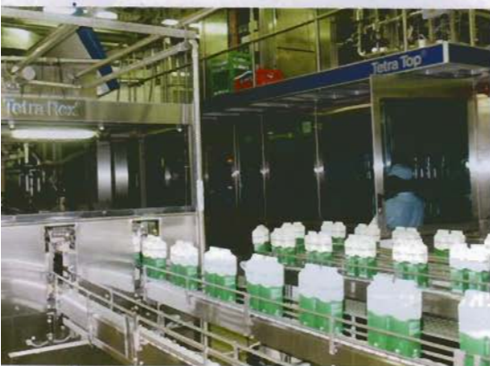
Fresh milk is filled by LM in gable-top cartons
