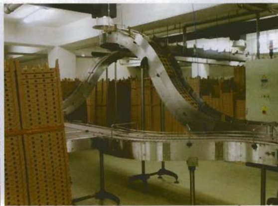
Carton trays are erected below the filling level and then transported directly to the machine
